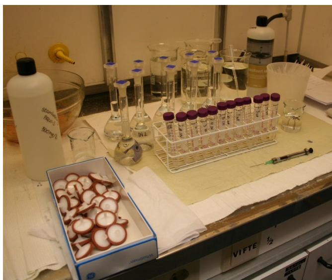
Figure 3. Standard and sample preparation for measurement of AQUI-S concentration
